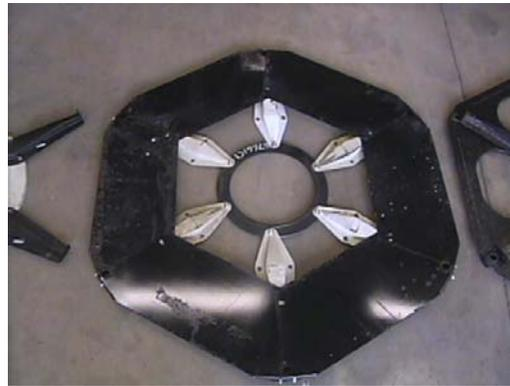
2. On top of the spider arm install one of the 7/8 I.D. (small hole) poly bushings to the arm with the 1/4” x 3 1/2” hex head bolts and locknuts. Again, only finger tighten these bolts.
